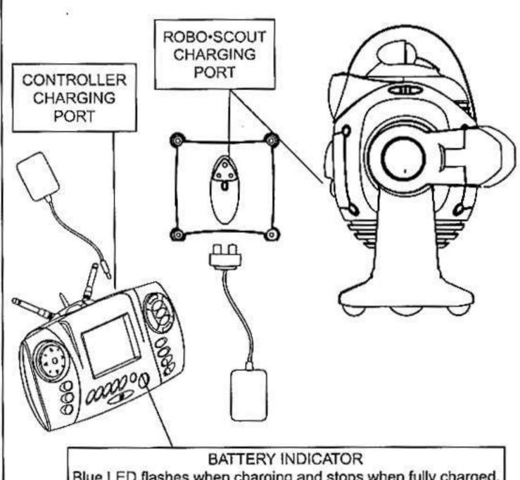
Blue LED flashes when charging and stops when fully charged.
