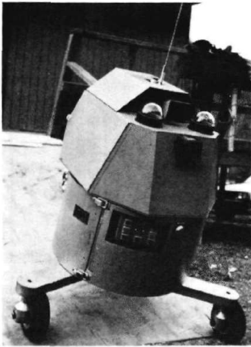
This radio-controlled robot called "Kluge" was designed for surveillance and to carry different types of equipment. (Credit: Cybernation Inc.)
