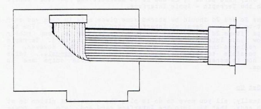
Now plug the card into slot 7 in the computer. As you stand in front of the computer, this is the last slot on the right. The side of the card with the ribbon attached to it should face the right wall of the computer. There is an opening in the back wall of the computer behind slot 7. You should be able to slide the ribbon into it as you lower the card into place. Again, although one must exercise caution not to bend any components, it requires some firmness to get the card into the slot.
