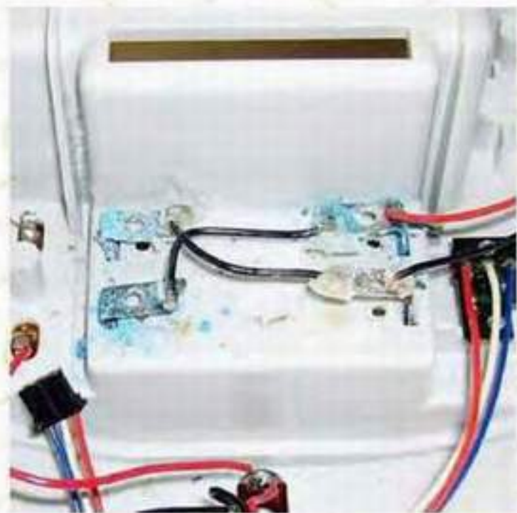
7. Gently pry the battery contacts out.
