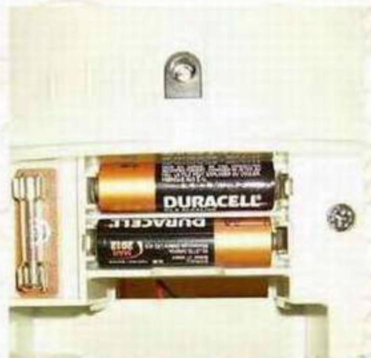
14. Install batteries into the robot housing.
