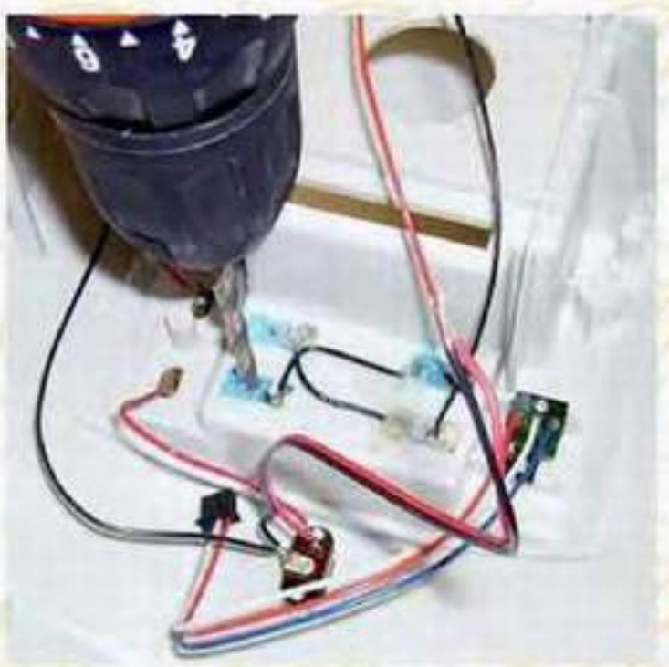
3. Place the housing flat on the table. Use a oversize drill bit and lightly drill the rim off the eye lit that hold the battery contacts in place.
