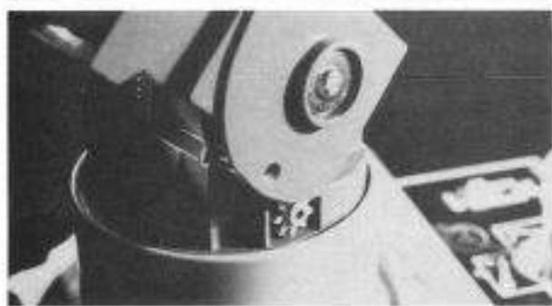
Photo 4. Close-up view of shoulder joint with decorative cover removed.
