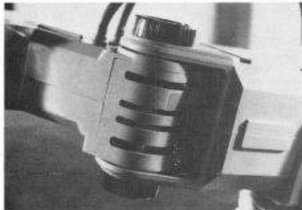
Photo 5. This view of the elbow joint shows the four gears used to provide motion from elbow to hand. Figure 7 explains each gear.
