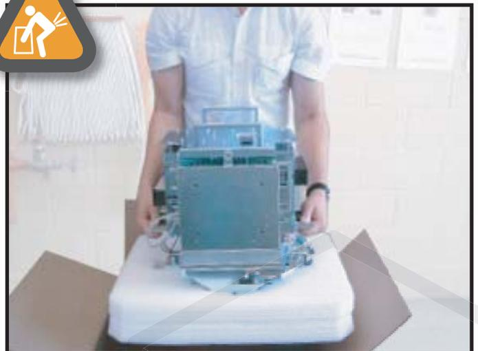
Lift the robot straight up out of the box. The foam base will come with robot as it is attached snugly.
