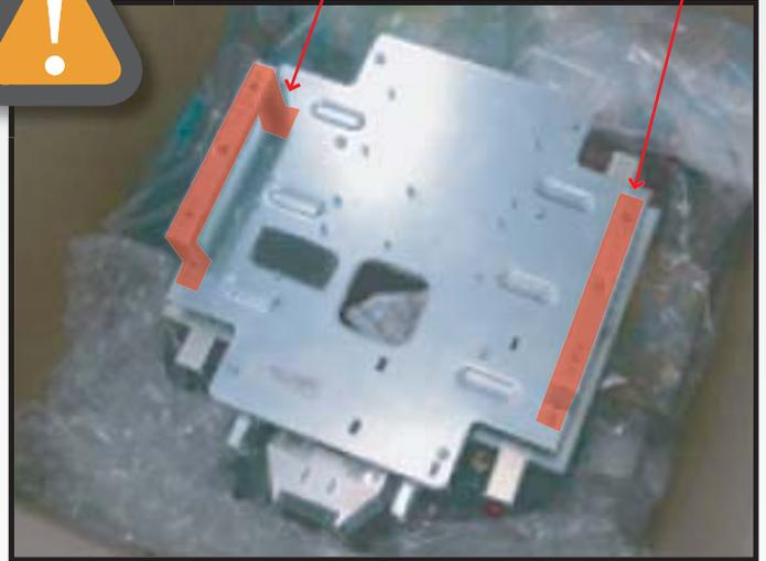
The handles are **NOT** the metal brackets visible on the top of the robot in the above diagram. The proper handles are located lower on the robot's body at the bottom of the drive bays.
