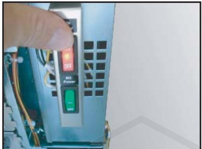
Switch on the Main Power switch on the front of the robot. **WAIT 5 seconds** and the M2-ATX Power Supply will cycle the power to the PC automatically.
