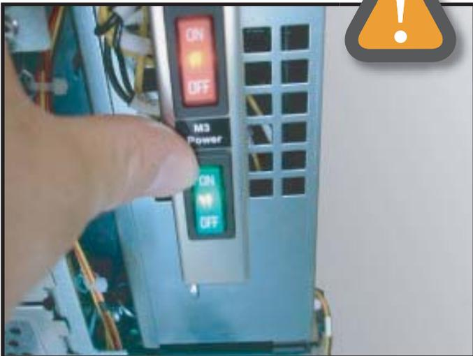
Next turn on the M3 Controller power. If this switch is OFF the M3 will not be able to drive the motors or read the sensors.
