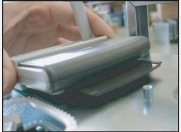
The Linksys Wireless USB Adapter has a mounting plastic plate on the top of the robot. The device which is in the box can slide onto this plate as shown.
