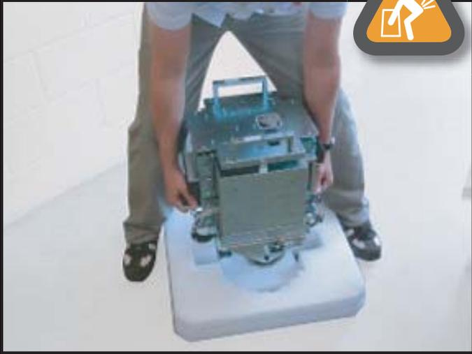
Place the robot down on the ground, with the foam still attached. Either hold the foam with your feet or have someone hold the foam while you pull the robot free.
