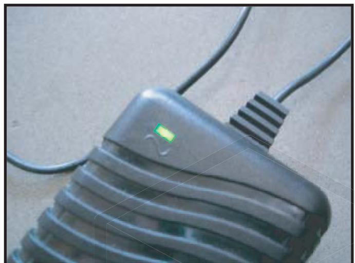
Once the charger is plugged into the robot, the LED will change from GREEN to ORANGE while it is charging. When it is finished it will switch back to GREEN.
