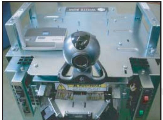
The Logitech Web Camera can be placed on top of the robot. Both will have to be plugged into the USB either on the CD-ROM/HDD holder or on the back of the Mini-ITX.
